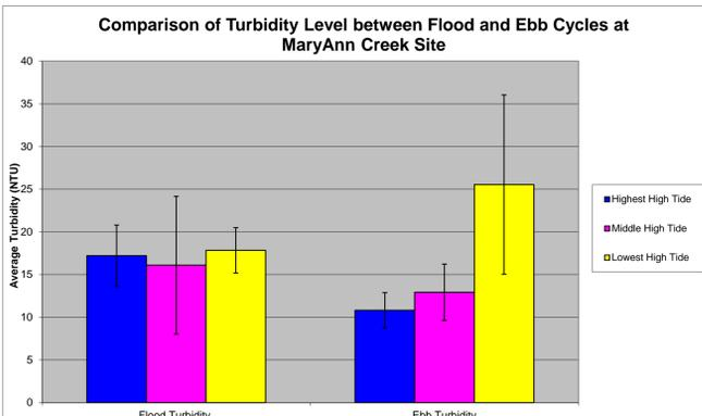
Average turbidity is generally greater in the flood phase than in the ebb phase, indicating that sediment is being brought into the creek. Sediment allows the marsh to accrete and keep up with sea level rise, and replenish vital nutrients
