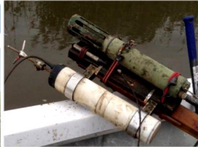
Left: A view of the sensor cluster measuring velocity, turbidity, and depth is ready to be deployed.
