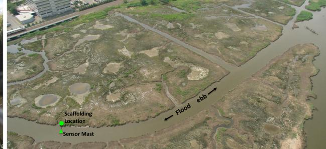
Above: Aerial image of Anderson Creek Site. Note the natural retention areas surrounding the creek that constitute the accommodation space. Hydro-flattened aerial LiDAR was used to survey the study area to determine proper placement of the sensors after each creek was selected.
