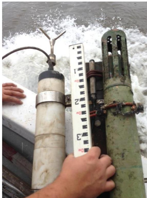
Figure 17 Sensor cluster from left to right: Sontek Argonaut 3 beam down looking ADV, CS451-L pressure transducer, YSI 6600 Multi-parameter Sonde
