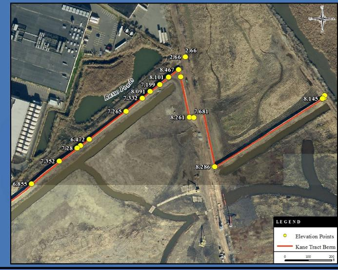
A berm constructed in 2010 within the Richard P. Kane mitigation site was overtopped by the Sandy storm surge. Field work was conducted to collect GPS elevations from the top of the berm and the resulting data complimented MERI water sensor readings. It should be noted the structure is not intended for flood control.
